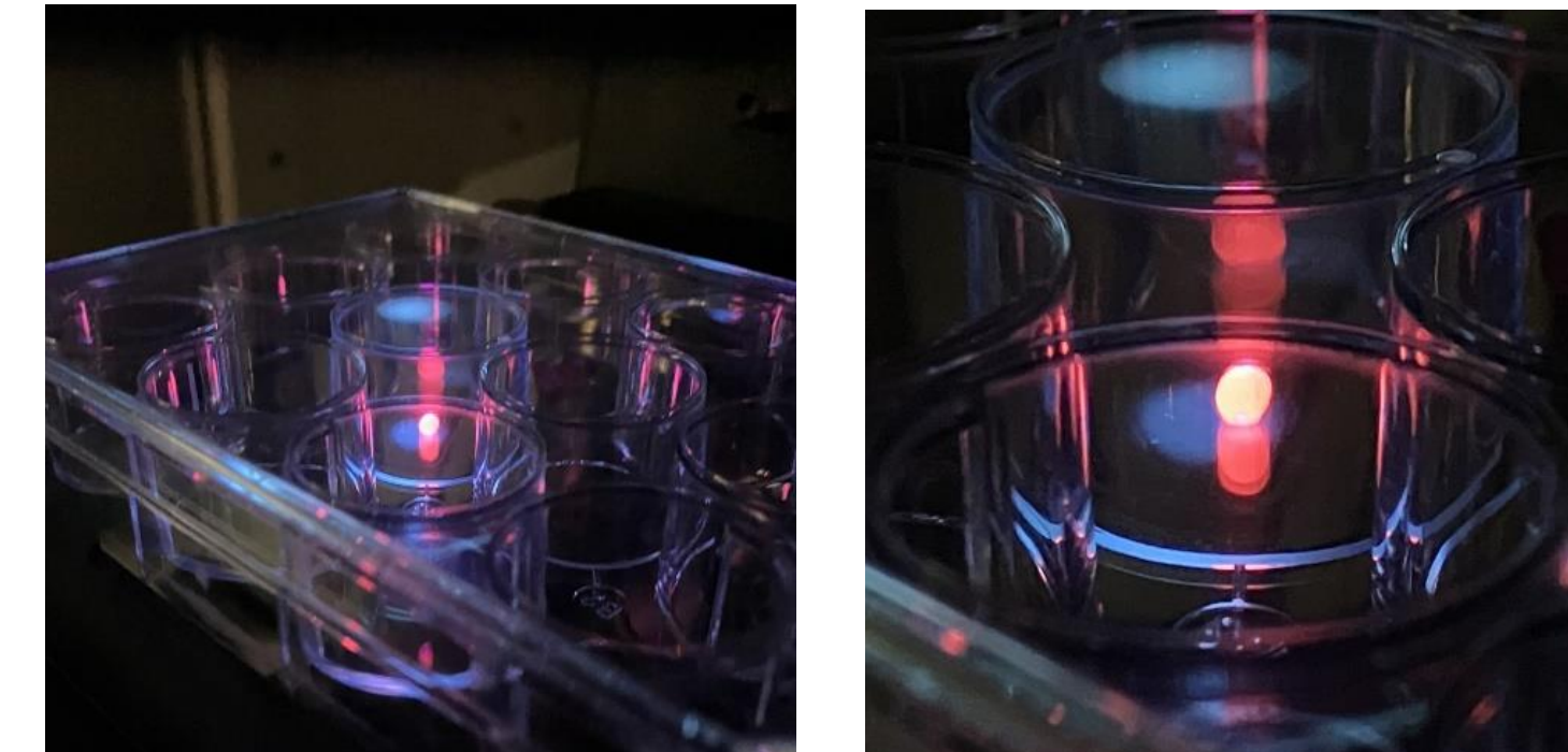
Fig. 6. Doxorubicin-loaded gadolinium-alginate exhibiting fluorescence under blue light displays high loading capacity for doxorubicin and viability as a fluorescent agent.
