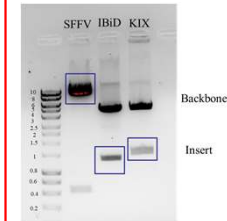
Figure 6: 1% Agarose gel: DNA separated backbone from inserts. Boxed in blue is where we cut the gel using a UV tray. Cut out SFFV backbone and IBiD and KIX inserts.
