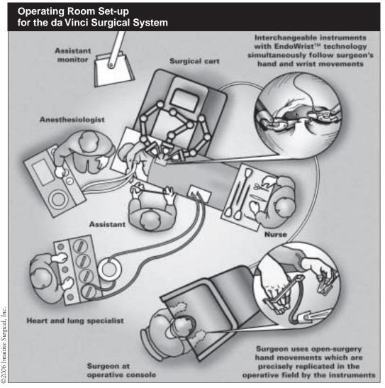
A short distance from the operating table, the surgeon views a highly magnified, three-dimensional image of the surgical site at a console. Here, **Dr. Surena Matin** demonstrates the controls which translate the surgeon's movements with better-than-human precision inside the patient.
